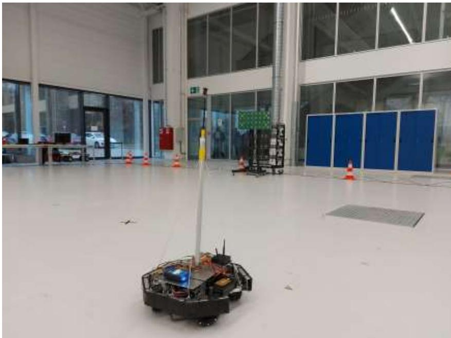
**Fig. 2: Left: Setup for channel measurement campaign in industrial environment (research factory “Arena 2036”) with robot-mounted mobile transmitter and 32-antenna array in the background.**
